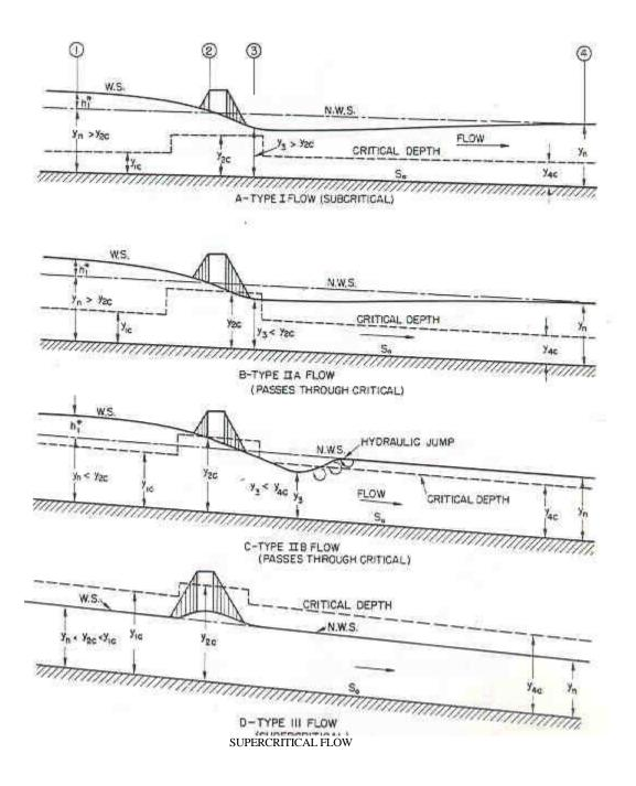
Figure 4 Types of Flow Which May Occur At a Bridge Constriction.
