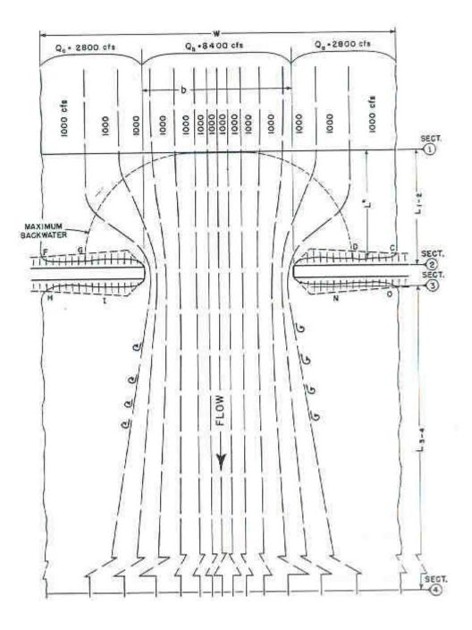
Figure 1 A Typical Pattern of Converging and Diverging Flow Lines That Occur at a Bridge that Causes a Constriction To the Flow
