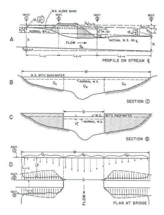
Figure 2 Schematic representation of how bridge backwater is measured <u>at the approach section</u> for a bridge with wingwall abutments
