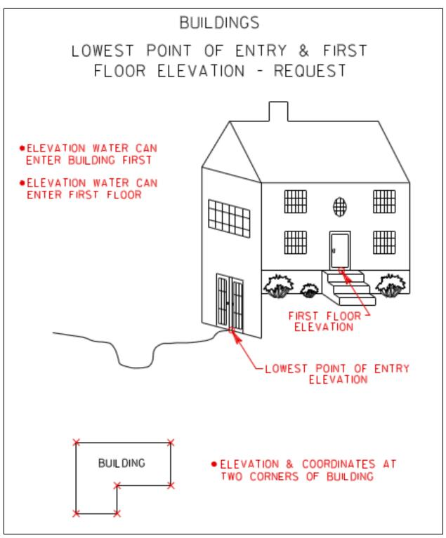
Figure 5-5. Survey Data Requirements for Buildings Potentially in the Floodplain
